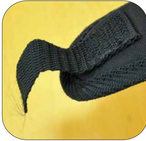
WEBBING NOT TAKEN INTO SEAM SUFFICIENTLY
