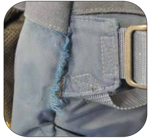
BROKEN SEAM. SEAM ALLOWANCE UNDER SPECIFICATION
