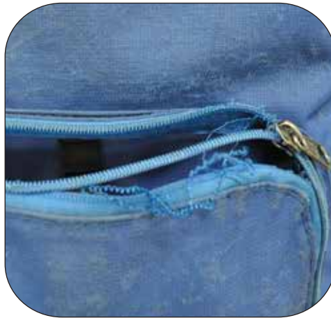
SEVERE DRAGGING / SCUFFING - MISUSE
