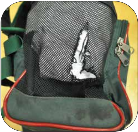
CUT / TORN MESH - MISUSE
