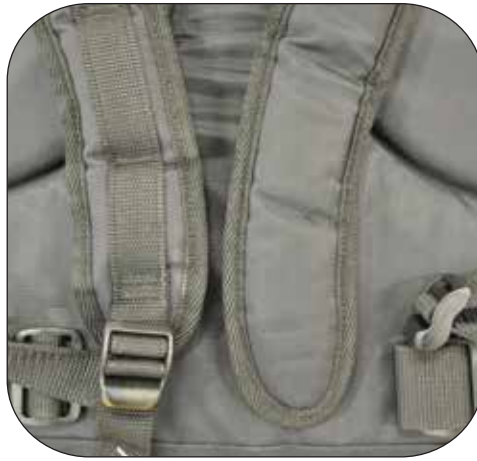
BAR TACK STITCHING ON SHOULDER STRAP MISSED IN PRODUCTION
