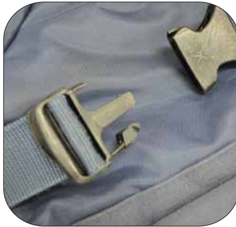
BROKEN BUCKLE - MISUSE
