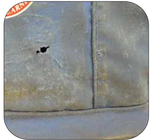
SEVERE DRAGGING / SCUFFING - MISUSE
